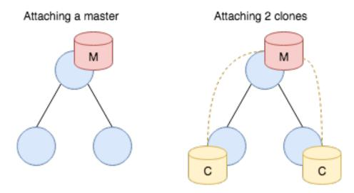
While the master can apply mutating operations to the store directly, clones have to first send the operation to the master and wait for the replay for the operation to take on effect:
