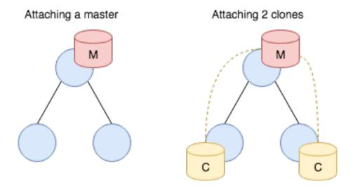
While the master can apply mutating operations to the store directly, clones have to first send the operation to the master and wait for the replay for the operation to take on effect:
