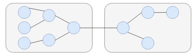
A process hosts one or more endpoints. Endpoints can communicate within or across processes as well as machine boundaries.
